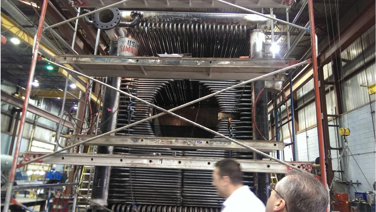
**Boiler #2 Replacement – Isometric View**
